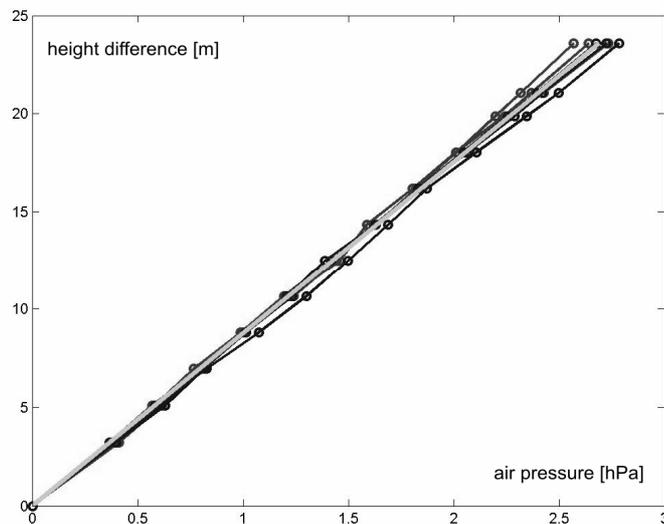
**Fig. 3.** Linear characteristic curve of six observations in our office building between the ground floor and the roof (6<sup>th</sup> floor)
